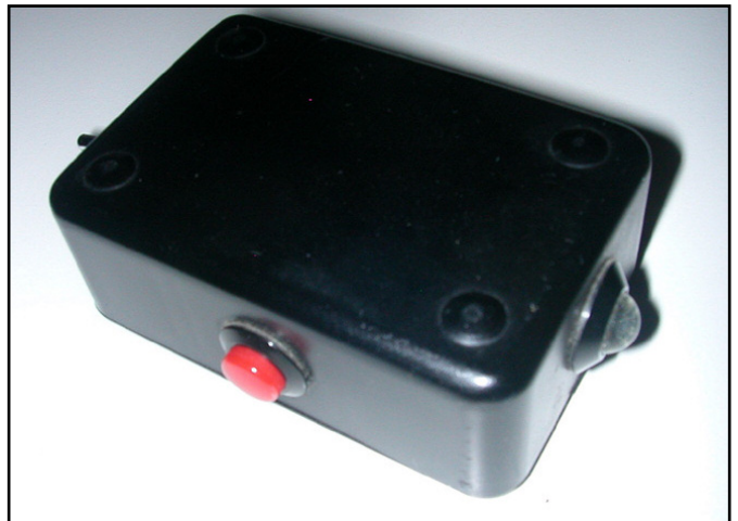
Photo A: The KI6SN version of the Trail-Friendly/Eye-Friendly Service Light is built into a plastic RadioShack project box — small and light enough for T-FR use and big enough so it won't get lost in your backpack. (Photographs courtesy of KI6SN)
