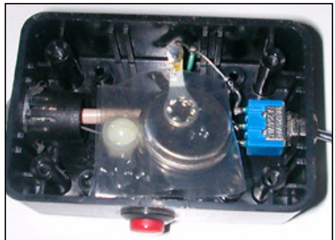
Photo B: A small plastic sleeve was crafted to hold the 3-volt lithium battery used to power the T-FR nightlight.
