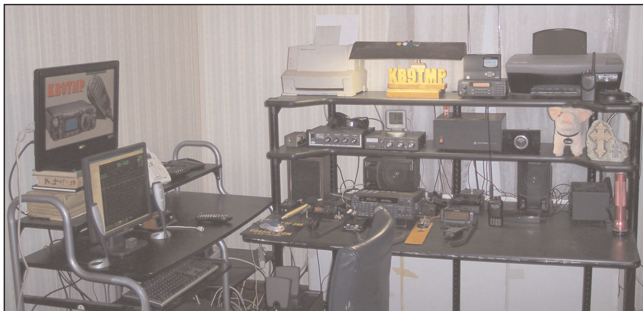
Photo A: From left on the desktop is KB9TMP's Yaesu FT-817 QRP transceiver, a Kenwood TS-450Sat HF radio and a Kenwood TM-V708a for 2-meter 70 cm. On the shelf above is a B&W VS300A tuner, a Yaesu FC-700 tuner and an Astron RS35A power supply. (Courtesy of KB9TMP)
