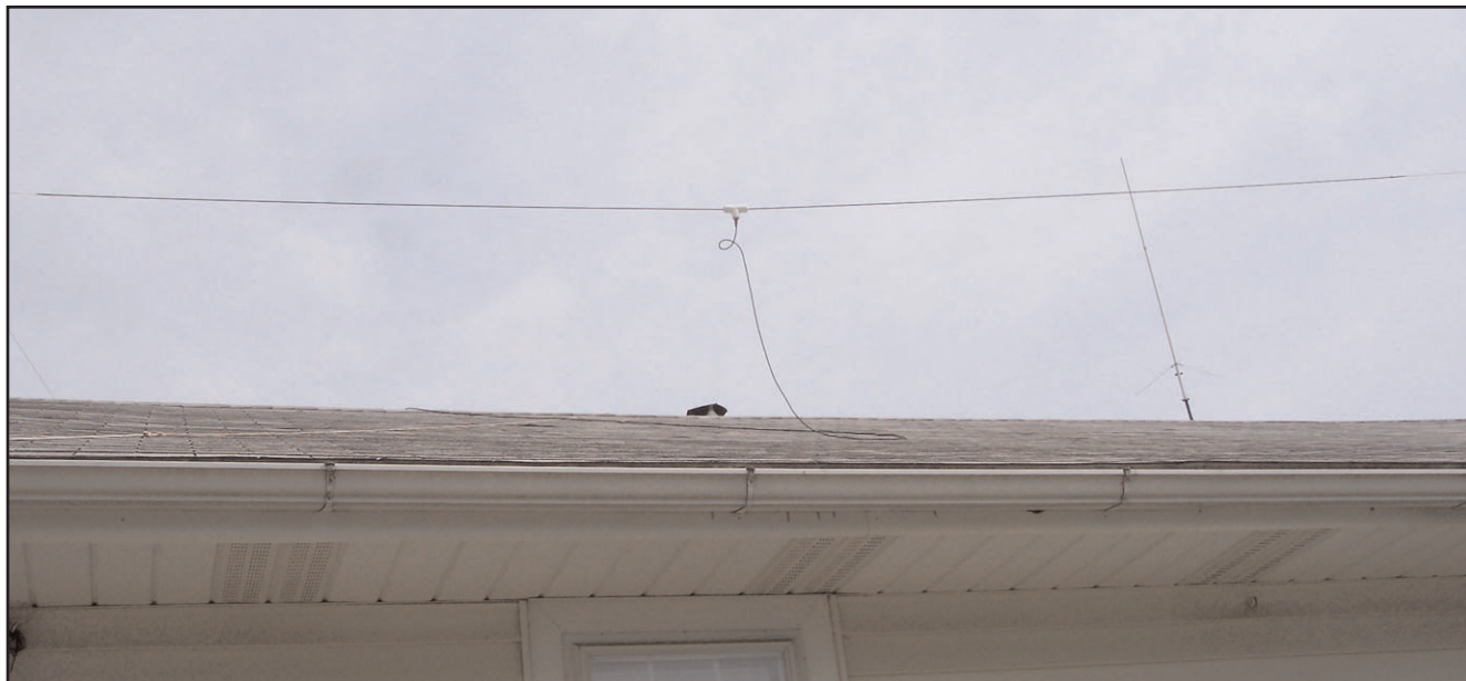
Photo B: KB9TMP's homebrew 20-meter double bazooka wire antenna with a Jetstream 2-meter, 70-cm vertical in the background.
