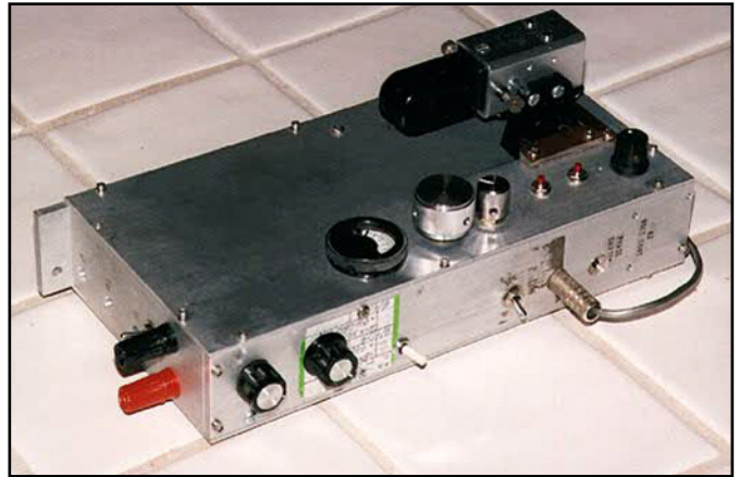
CQ Amateur Radio magazine’s QRP columnist Cam Hartford, N6GA, designed a trail-friendly, contestworthy radio in the mid-1990s that would become one of the inspirations for Elecraft’s renowned KX-1 T-FR transceiver. (Courtesy of KI6SN)
