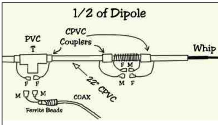
Place a CPVC coupler onto the other side of the coil. Place the piece of CPVC that holds the telescoping whip into the CPVC coupler to the coil. Note that there is a male electrical connector on the coil. This attaches to the female electrical connector on the whip assembly. This completes the antenna assembly. (SEE PHOTO ... drawing)
