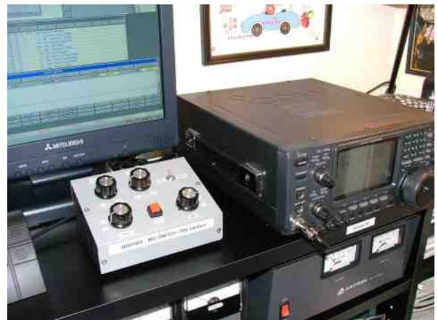
This switch can be custom made for any type of radio; the enclosure can be any style but feel you should use solid metal for RF Shielding.
