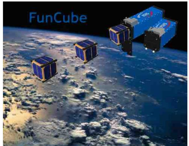
FUNcube will carry a UHF to VHF linear transponder that will have up to 1 watt and which can be used by Radio Amateurs worldwide for SSB and CW communications. Measuring just 10 \* 10 \* 10 cm, and with a mass of less than 1kg, it will be the smallest ever satellite to carry a linear transponder and the choice of frequencies will enable Radio Amateurs to use their existing VO-52 or DO-64 station.
