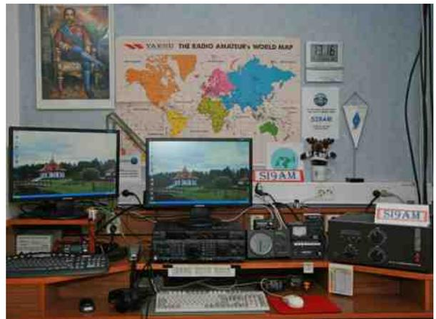
The station equipment consists of an FT 1000 MP with an ACOM 1000 amplifier. A 24-meter mast holds a tribander beam for 10/15/20 meters and a two-element for 40 meters. For other bands there are various wire antennas. A number of different software like TR, DX4WIN, HAM-Log, WIN-TEST and others is used for logging.
