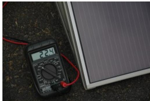
*Shown here is the no-load output voltage (on the small DDM) in an almost clear sky. As you can see, the no-load voltage is around 22VDC. This drops to about 14-15 volts under load*
