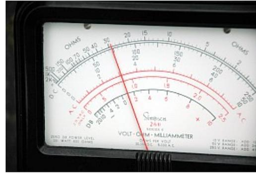
*My 40 year old Simpson 260 Multi-meter shows just a hair under 3 A when placed directly across the three PV panels in parallel. This equates to about 45 W total output UNDER FULL SUNLIGHT*
