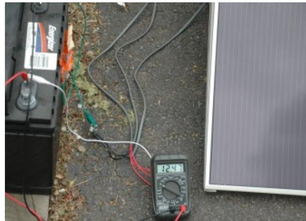
*The final product: the 45W PV system is charging a deep cycle battery used in our Scamp camper. Notice that there is no charge controller and the reason for that is, this system won't really overcharge this battery even if left for an extended period.*
