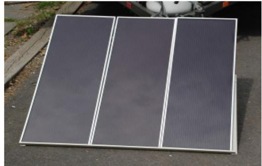
*This is the overview of the Harbor Freight 45 W solar power "kit". Each PV is 15 W, when combined in parallel they provide approximately 3A at 14-15VDC output for battery charging.*
