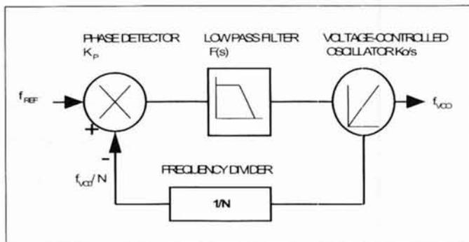
▲ Figure 1. Block diagram of a PLL.
