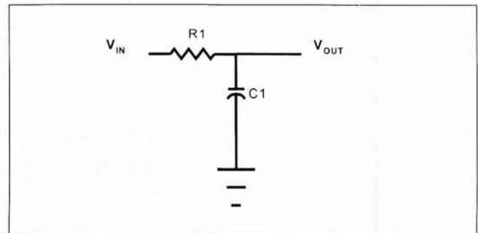
▲ Figure 4. Single pole loop filter.
