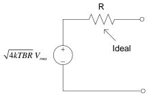
We can now ask: What is the maximum available noise power from this noisy resistor? To determine this, we'll attach a <u>perfect</u> (i.e., noiseless) resistor R to this circuit [Fig. 14.1(b)]:
