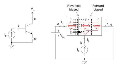
The EBJ is forward biased and electrons are injected into the p region just as with a forward biased diode.
