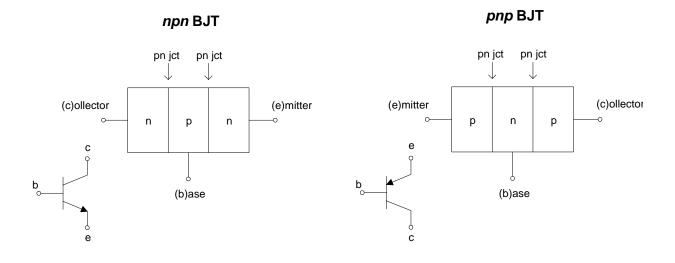
BJTs actually look a bit different than this when manufactured. Most importantly, they are usually not symmetric devices.
