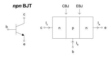
Measuring the dc resistance from c to e would indicate a very large value since we have two back-to-back *pn* junctions. This
