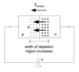
The electric field produced by the battery  $E_{\text{battery}}$  adds to the electric field of the space charge *E* in the depletion region. This <u>increases the width</u> of the depletion region.
