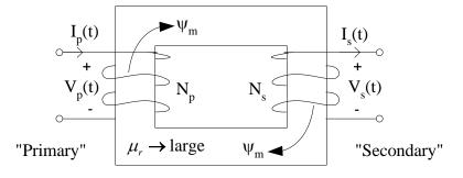
The time varying current  $I_p(t)$  in the "primary" circuit produces a magnetic flux density  $\overline{B}_p(t)$  in and around coil p. Similarly, the "secondary" coil produces  $\overline{B}_s(t)$ . The total magnetic flux density is the sum  $\overline{B}(t) = \overline{B}_p(t) + \overline{B}_s(t)$ .
