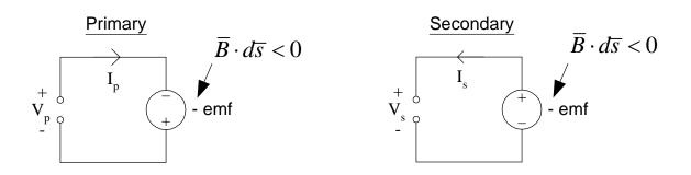
The polarity of the lumped *emf* source is set by the direction of the current: a voltage <u>source</u> has current entering the negative terminal. The sign of the *emf* source is due to the direction of  $d\overline{s}$  (by the RHR) and the assumed direction for  $\psi_m$  (and hence  $\overline{B}$ ).
