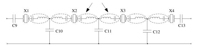
The next step is to recognize the presence of impedance inverters positioned between each quartz crystal.
