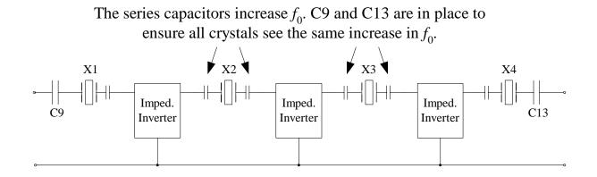
What remains are two capacitors in series with the crystals X2 and X3. We can now see that the purpose for C9 and C13 is to ensure that X1 and X4 also see the same capacitances.
