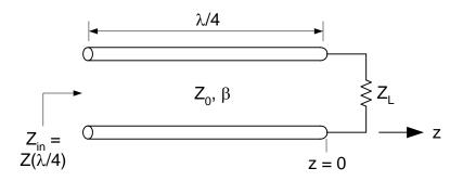
Recall from Lecture 9 that for an open circuit load  $(Z_L = \infty)$ ,  $V(\lambda/4) = 0$  and  $I(\lambda/4) =$ maximum. Therefore,  $Z(\lambda/4) = 0$ . Consequently, this TL has "inverted" the load impedance.
