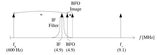
One difficulty here is that the BFO image is only about 1.2 kHz away from the IF. For a center frequency of 4.9 MHz, we need a bandpass IF filter with a Q of approximately
