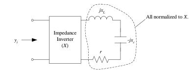
The impedance inverter, according to (5.41), provides a normalized input admittance  $y_i$  of
