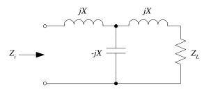
Notice that the magnitudes of the inductive and capacitive reactances are equal in this circuit. This strictly can occur only at a single frequency. So this impedance inverter will be a narrowband device, which is ok for us since the IF Filter will have a very narrow passband.
