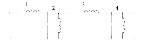
We can recognize this equivalent circuit as a fourth-order, bandpass LC ladder filter! Consequently, this fourth-order Cohn filter using quartz crystals is *effectively* a fourth-order, bandpass LC ladder filter.
