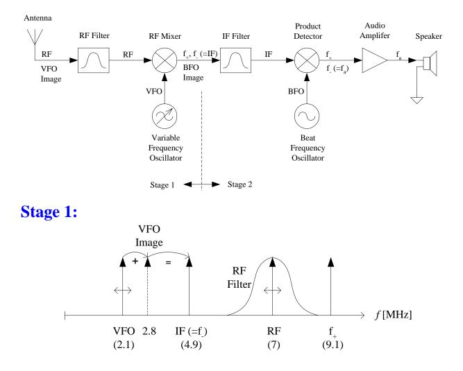
After this, the IF signal is mixed with the BFO signal by the Product Detector down to audio frequencies (approximately 620 Hz in the NorCal 40A).
