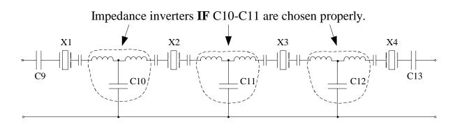
Replace these tee networks with impedance inverter circuits:
