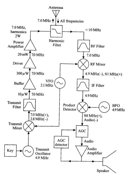
**Figure 1.13.** Block diagram for the NorCal 40A. Sum frequencies are noted by + signs, and difference frequencies by - signs. Adapted from Appendix C of the *NorCal 40A Assembly and Operating Manual*, by Wayne Burdick, published by Wilderness Radio. Used by permission.
