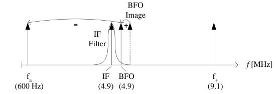
The IF Filter needs to have a very large Q. Its job is to filter out the sum frequency signal ( $f_+ = 9.1$  MHz) and the BFO image (if there is one at  $\approx 4.9$  MHz).
