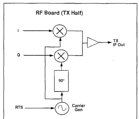
Figure 4. The transmit half of the WA4DSY modem. Since the design is modular, you can save the RF board in half to set up a completely independent receiver and transmitter section.
