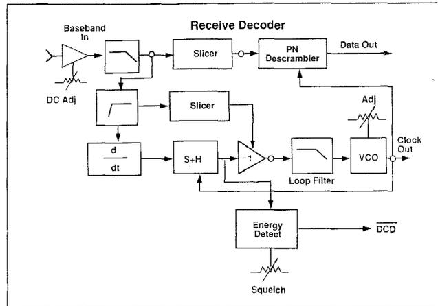
Figure 6. The receive decoder card adjustments are straightforward.
