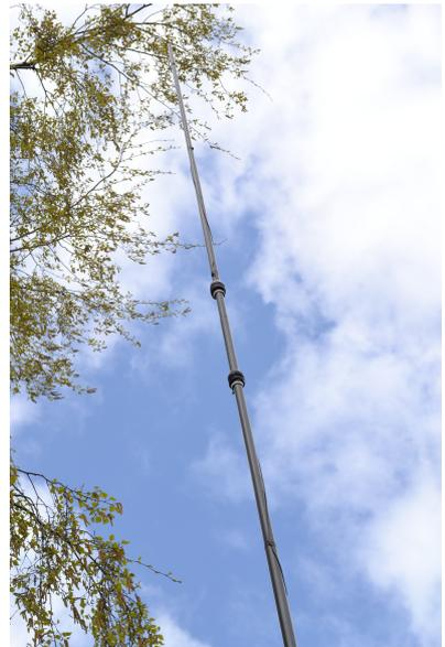
This actually makes sense as the end of an EFHW is at the same impedance as the end of a quarter-wave vertical, so a trap does the same thing. All you have to control is the resultant high feedpoint impedance. Doh! – why didn't I think of that earlier?
