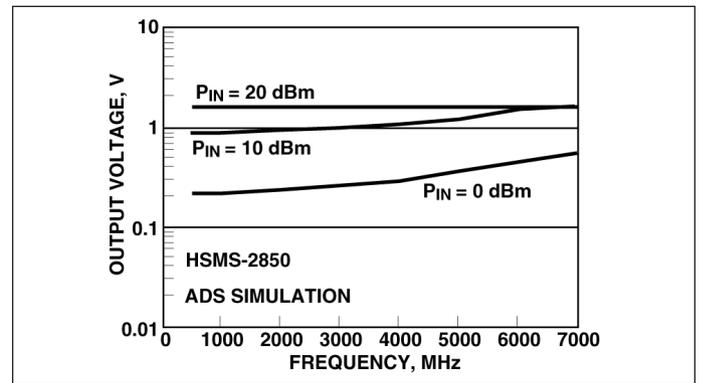
▲ **Figure 5.** Simulation of the HSMS-285x diode family of small-signal zero-bias detectors. Such p-type low-barrier diodes are characterized by series resistance and low breakdown voltage, causing the diode to saturate.
