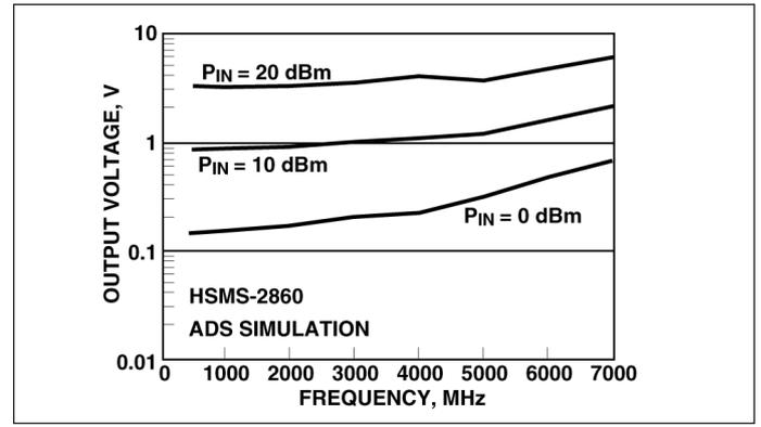
▲ **Figure 4.** Simulation of the HSMS-286x diode family showing improved performance above 4 GHz.
