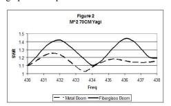
fiberglass boom related graphs are depicted with the solid lines. The results of my SWR evaluation were a bit unexpected. The overall SWR of both antennas is very good so I am not complaining, but there appeared to be no significant change in the SWR of the 2-meter antenna, and a slight degradation in the SWR of the 70-CM antenna.
