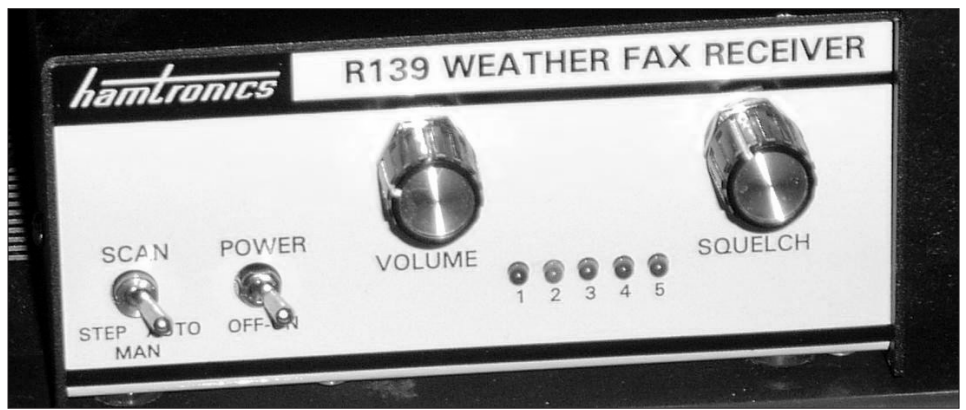
Figure 5: Example of a dedicated satellite receiver.
