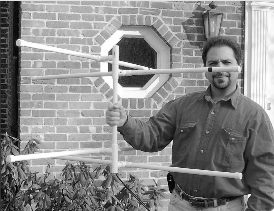
Figure 6: A simple, but effective, satellite receiving antenna can be made from materials purchased from your local home improvement store. The antenna is unobtrusive, lightweight and easily installed on a rooftop.
