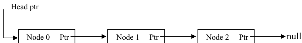
Fig. 49-2 Linked list using only forward pointing pointers (singly linked).
