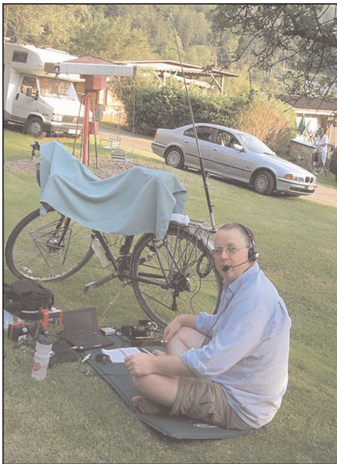
A base-loaded, ATX100, mobile whip antenna is mounted on the back of Dominic Baines, M1KTA’s, bicycle for on-air operation during a 1,100+ mile ride in Europe a year ago this month. (Photographs courtesy of M1KTA)
