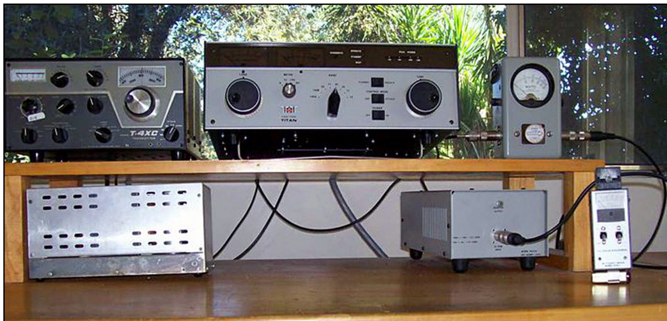
A Drake T-4XC transmitter, Ten-Tec amplifier, Bird wattmeter, Palomar Engineers clamp-on RF current meter and Ten-Tec dummy load were used in Kurt's skin effect experiment. (Courtesy of Kurt N. Sterba)
