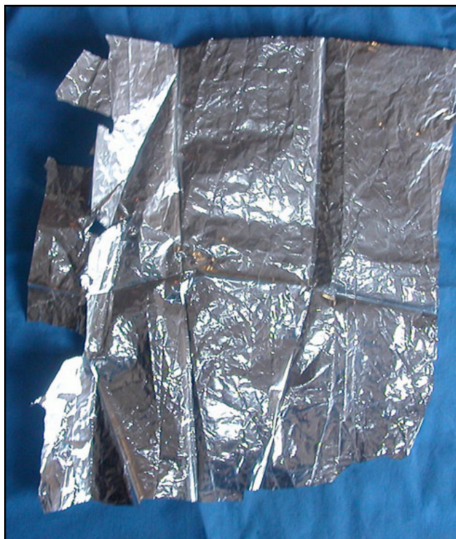
The 10-story tall ECHO-1 was made of aluminum-coated Mylar® just one-half millimeter thick – as this historic remnant from the sateloon construction cutting floor shows. (Courtesy of K16SN)
