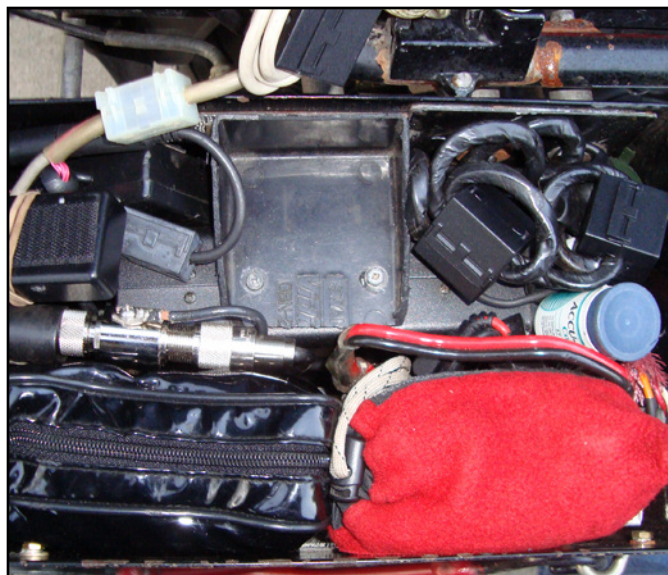
Fifty-caliber ammunition boxes on each side of the motorcycle carry all electronics, tools "and when needed, an extra battery for special events."
