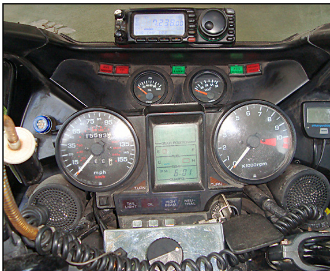
The control head for KA9PGC's Yaesu FT-100D sits protected behind the windscreen where "rain and snow are not a problem."
