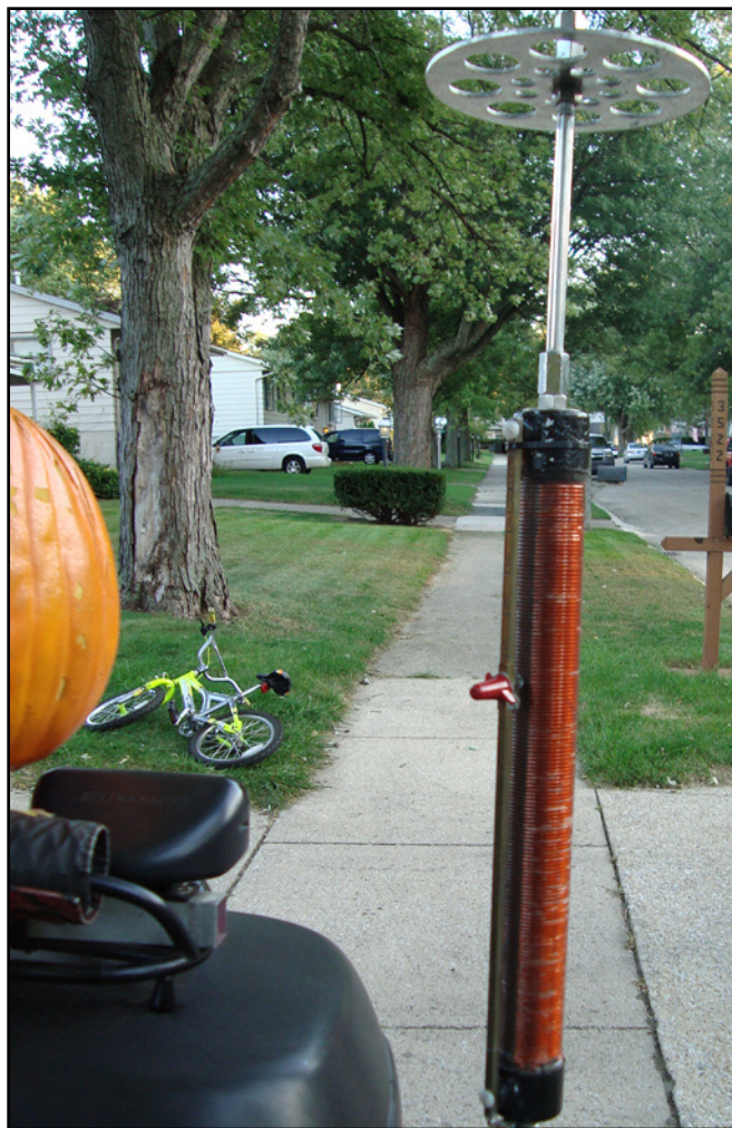
The low band antenna "is completely homemade and designed out of about 50,000 miles of experience. I describe it as an 'off center fed vertical dipole,'" KA9PGC says.
