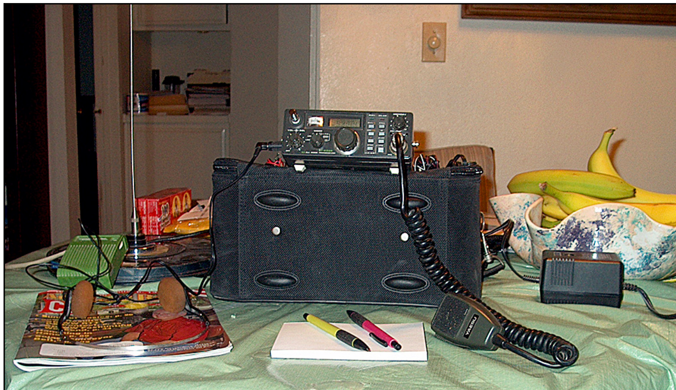
The portable "Go Kit" station set up and ready to go using the carrying case as a mount. The antenna is to the left in the background.
