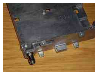
FT817 internal chassis
