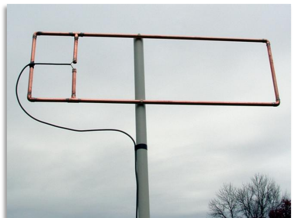
The Hentenna mounted for a vertically polarized signal.
