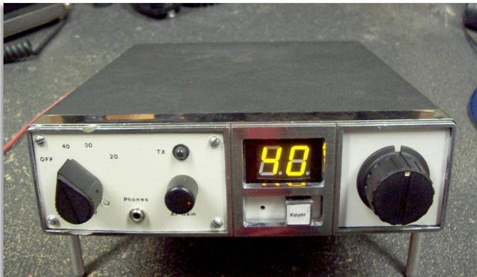
The "Multiwonder," A tri-band rig built into an old CB case. For more detail on this rig, see the March 2008 BBQ and visit http://geocities.com/n2uhc_3/multiwonder.html
