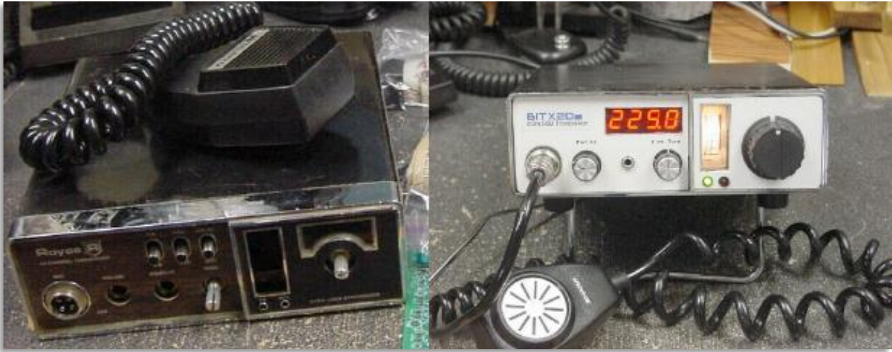
A before and after shot of a BitX20 built by Tom, N2UHC FP#-1149.
