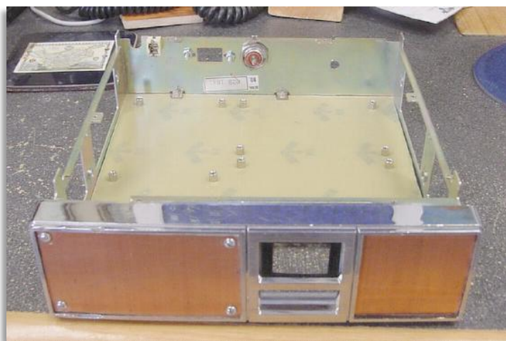
A CB case with newly-installed PCB front panels.
