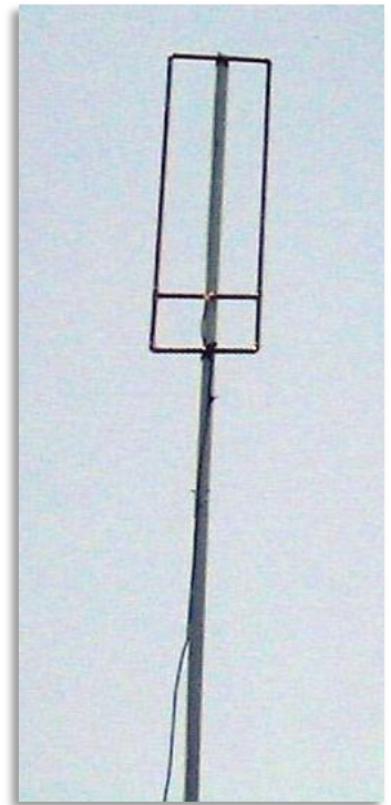
The Hentenna mounted for a horizontally-polarized signal
