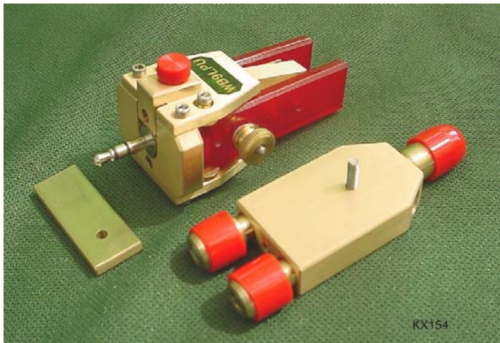
This is the paddle removed from the base. The legs have been stowed in the base, where they are held by internal threads.
