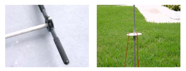
The picture on the left is the die that Tom used to cut the threads into the rod. The picture on the right shows two of the top sections put together with the couplings and the disc that we fashioned into a support for guying.
