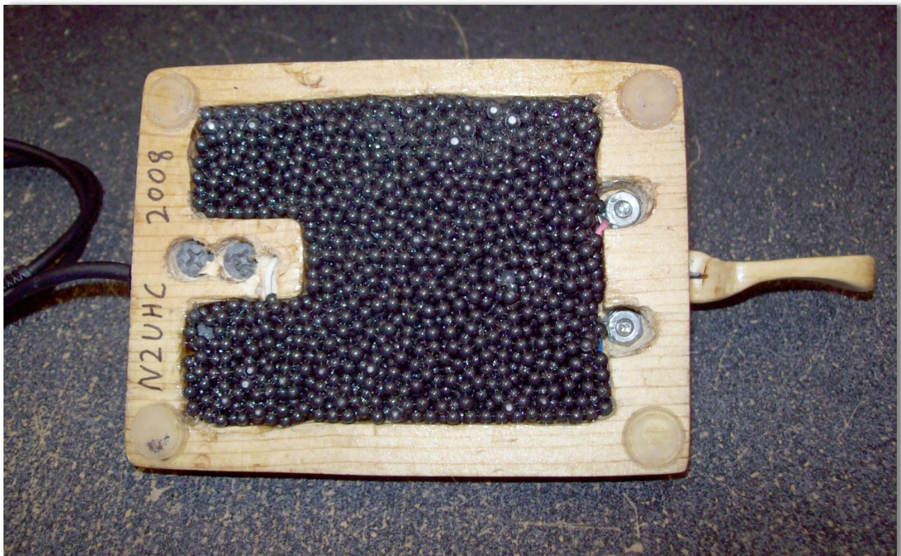
A detailed view of the bird-shot weighting of the paddle
